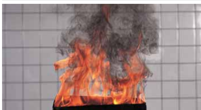
Test fire 5: liquid fire (n-heptane)
