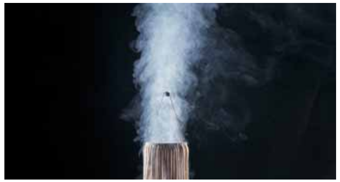
Test fire 3: glowing smoldering fire (cotton)
