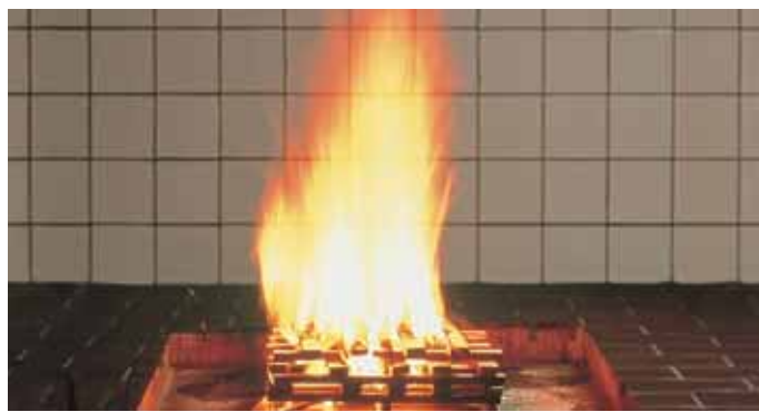
Test fire 1: cellulose open fire (wood)
